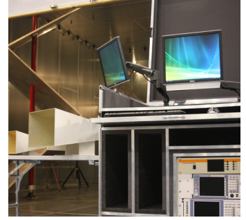
Our reverberation chamber can achieve test frequencies as high as 40 GHz
