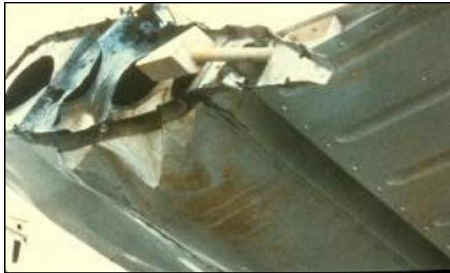
Figure 7. Example of severe stroke damage to small airplane wing tip (same damage occurred to opposite wing tip)
