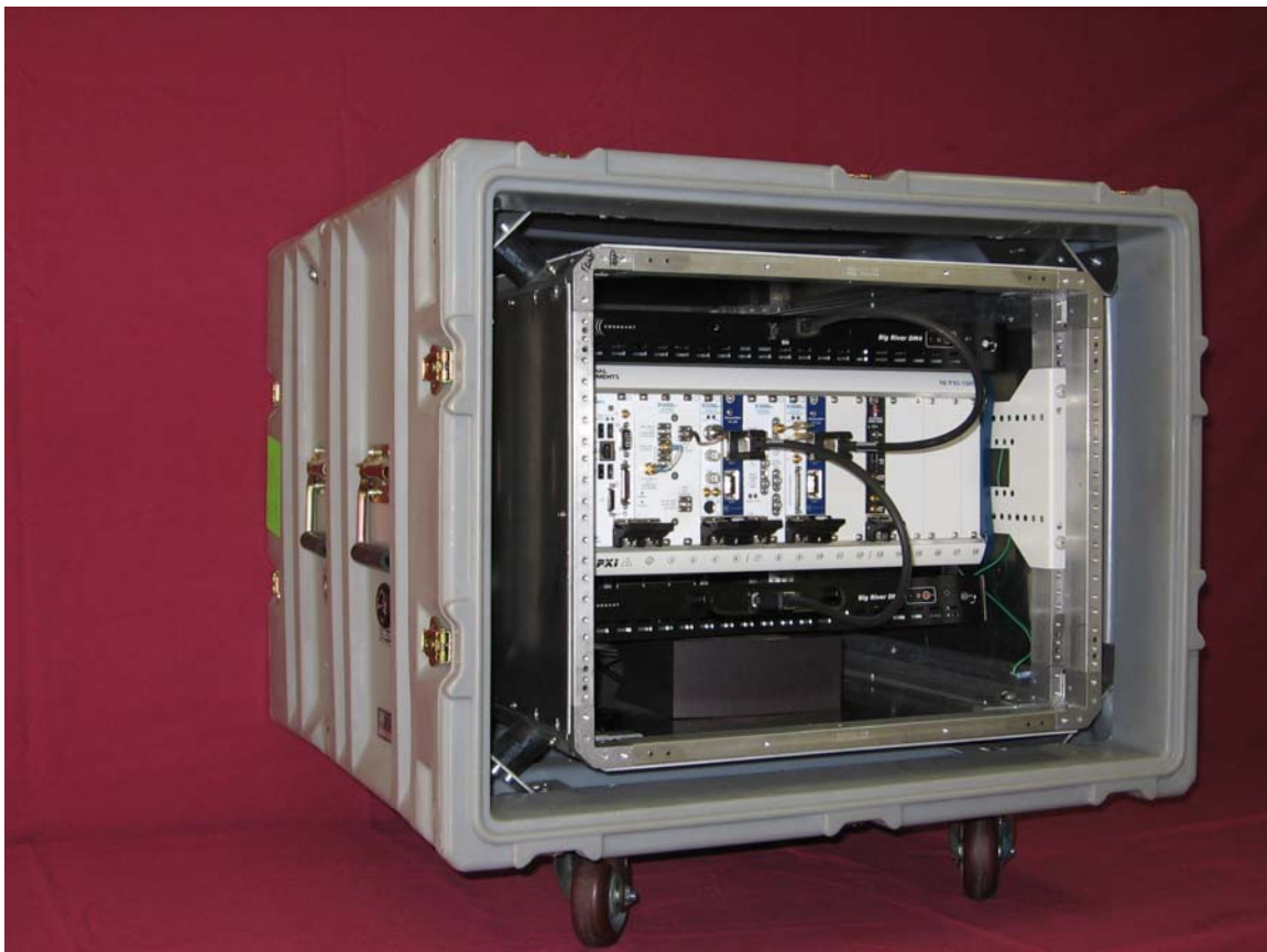
Portable version of a combination record and playback system with GPS
