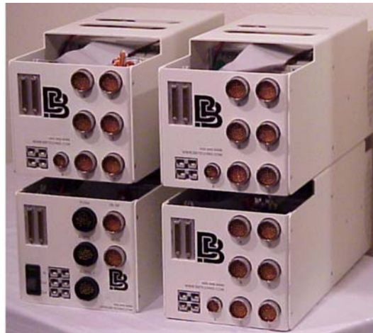
4 SCXI mainframes filled with thermocouple conditioning modules
