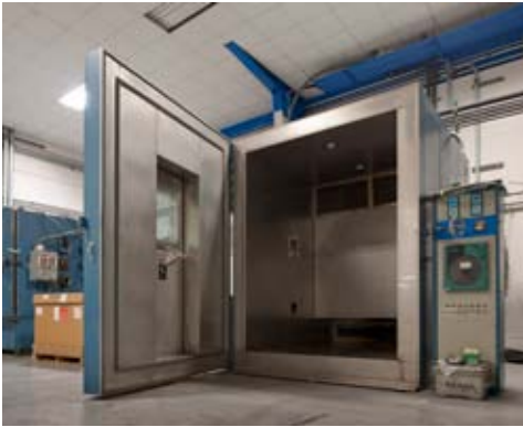
Walk-in chambers allow for temperature, humidity and combined environmental tests on large test specimens.
