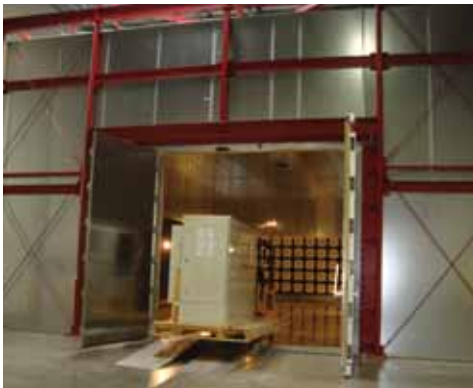
EMC/EMI test capabilities are available in many NTS facilities and include multiple shielded and anechoic chambers.
