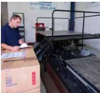
Dynamic shock, random and sinusoidal vibration detect possible product faults during the NEBS qualification tests.
