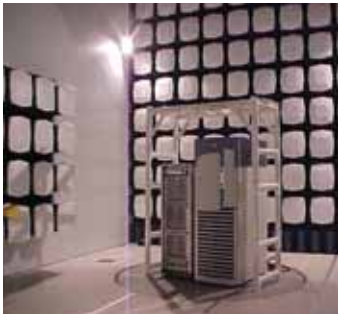
Complete system tests can be performed in any of the NTS anechoic chambers.
