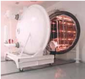
1500 cubic foot Thermal Vacuum Chamber
