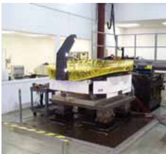
Cloudsat Spacecraft Radar Antenna undergoes Force Limited Vibration Testing
