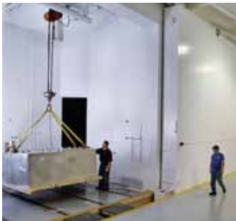
5000 square foot Acoustic Noise Reverberation Chamber
