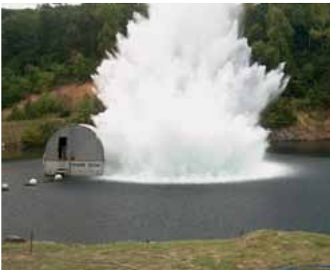
NTS's full spectrum test and research facilities are capable of managing your environmental test requirements, including MIL-S-901 high impact, heavyweight shock testing.
