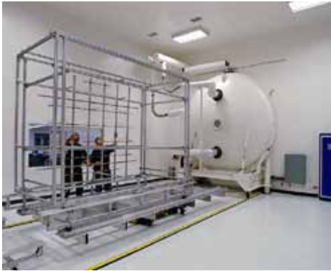
Special test environments are required to simulate space conditions in order to evaluate the life expectancy of today's communications and military satellites.
