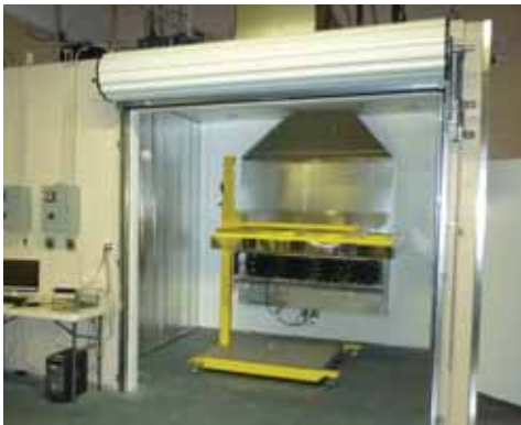
State-of-the-art solar radiation chambers can be configured to accommodate large or odd-sized test articles
