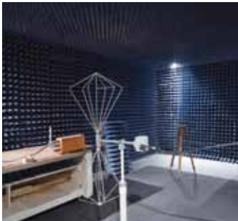
Shielded and anechoic chambers are on-site for emissions and susceptibility testing
