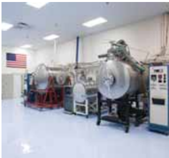
Space simulation capabilities include thermal vacuum cycling from -180°C to +180°C with TQCM monitoring
