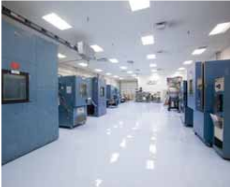
A large selection of climatic simulation chambers accommodate small to very large test articles
