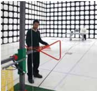
Radiated Emissions testing conducted in our 10-meter semi-anechoic chamber.
