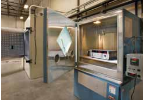
Temperature testing conducted in our Environmental and Dynamics laboratory
