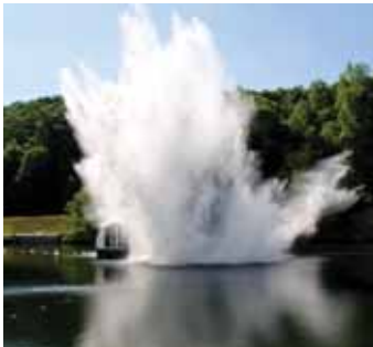
MIL-S-901 Heavyweight Shock Testing
