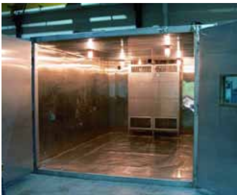
Walk-in chambers can accommodate large equipment and heat load
