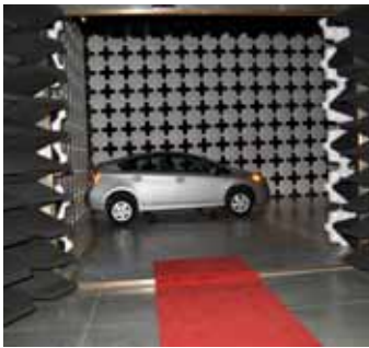
Testing in new 10-meter EMI chamber
