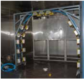
NTS preparing a solar-load test set-up
