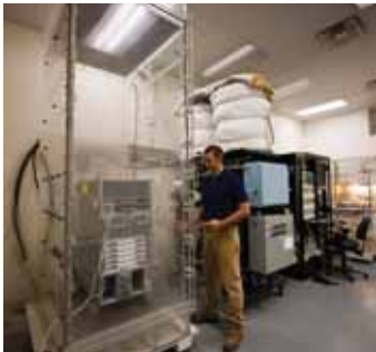
Mix Flowing Gas (MFG) testing environment
