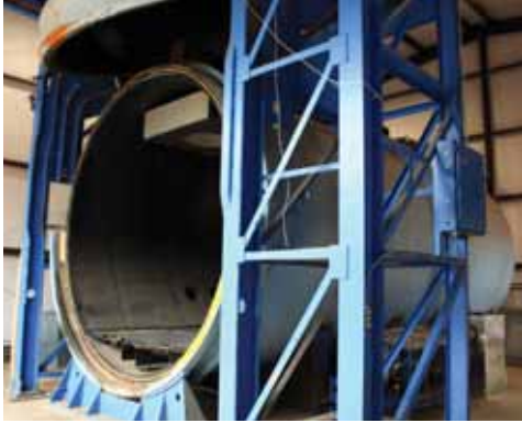
Our 11'x26' temperature/humidity/altitude chamber is capable of reaching temperatures from -80° to 170° F and simulating altitudes of up to 90,000'
