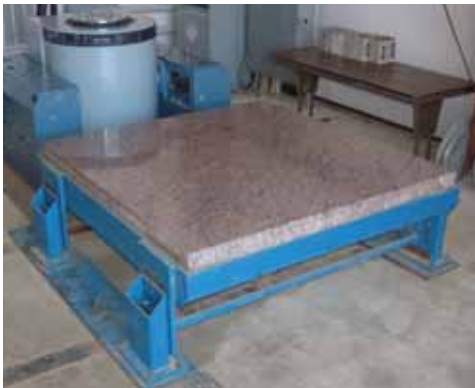
Multiple electrodynamic vibration systems are available, with stroke capabilities up to 3" and force capability up to 40,000 force pounds
