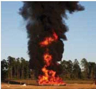
MIL-STD-2105C fast cook-off test being performed on high-explosive warhead
