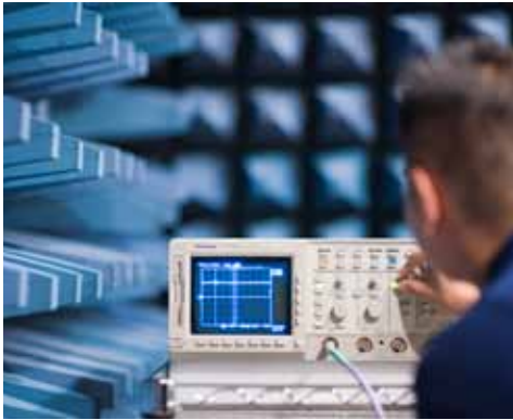
Semi-Anechoic Chamber for Radiated Susceptibility Testing
