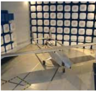
UAV Testing in EMI Chamber
