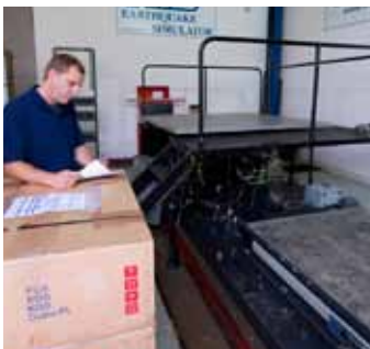
Seismic (Earthquake) Testing 3-Bay Rack Holds up to 3,500 lbs
